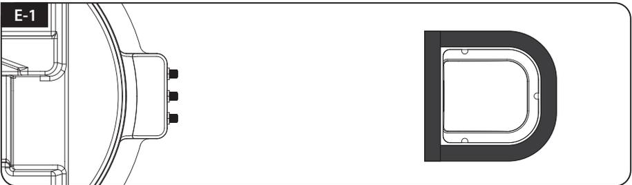
Place cable holder around 30CM from the rear centre of the antenna. Apply friction tape 5mm from the outside of the holder
